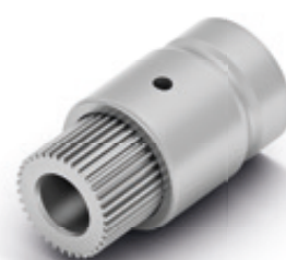
DESIGN WITH INTEGRATED COUPLING With continuous gearing, the coupling toward the gearbox serves as axial stop and sealing element at the same time.
