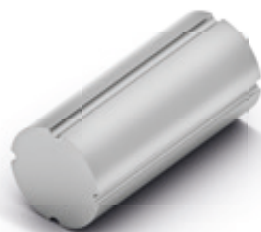
ROUND SHAFT WITH HALF-ROUND SLOTS Up to four round keys transfer the force. The key can be integrated in the screw element.
