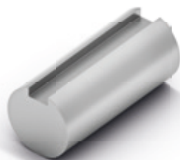
ROUND SHAFT WITH FEATHER KEY Used only rarely now because of the limited permissible torque.
