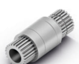
THREE-PIECE DESIGN The gearing of the traversing range is continuous where the dual-gear drive element as well as the stop and sealing element is pushed in place in sleeve-fashion and secured with a bolt from the drive side.
